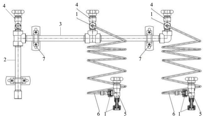
Manifold M 3302 for 2 cylinders with left side connection
