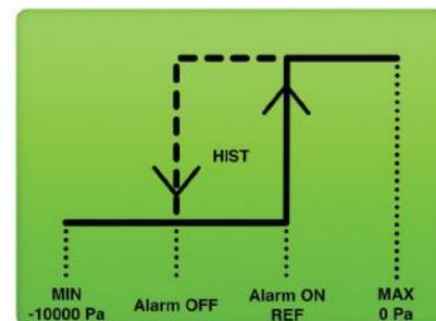
The alarm is activated when the vacuum is higher than reference. Alarm is released when vacuum is lower than reference plus value of hysteresis. Factory pre-set is -0.2 bar (-20000 Pa) (pull up)
