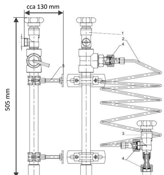
Wall adapter M 3311 for 1 cylinder with left side connection
