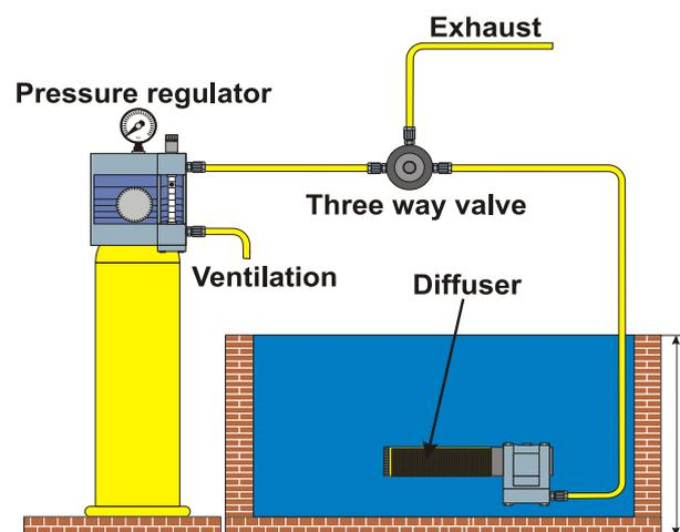
Principle of installation of the pressure regulator
