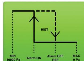
The alarm is activated when the vacuum is lower than reference. Alarm is released when vacuum is higher than reference plus value of hysteresis. Factory pre-set is -0.5 bar (-50000 Pa) (pull up)
