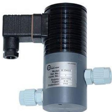
**Solenoid (Electromagnetic) valve** is designed to operate in chlorine gas lines under vacuum. It is designed to shut off vacuum between ejector and chlorinator (vacuum regulator). Valve is normally closed and opens only when power is applied. At power loss the valves closes and cuts off vacuum to the system.
