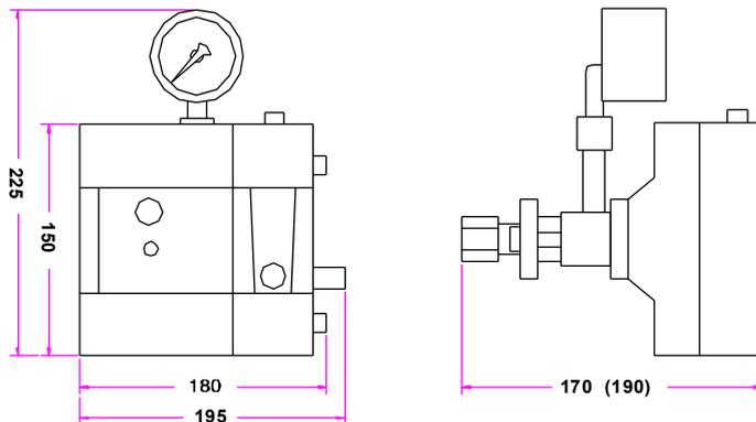
**Attention!** Dimensions in brackets are dimensions of vacuum regulator equipped with pressure gauge!
