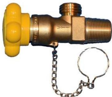
**Chlorine cylinder valve** made with O-ring sealing system and spindle thread outside gas wetted area. Valve seat and lower spindle are made of stainless steel, upper spindle is made of brass.
